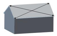
If the roof is not square, follow the 3-4-5 method to ensure that the panel is being installed square. If the first panel is not installed square, all remaining panels will also be out of square when attached to the structure.
