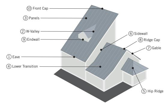
Installation over shingles is possible but is not recommended. It is best to remove shingles and install a new, synthetic underlayment to act as a vapor barrier between the substrate and the metal. If shingles will not be removed, furring strips need to be installed on the roof at 2'-0" centers. The metal panels will then be fastened to the furring strips.
